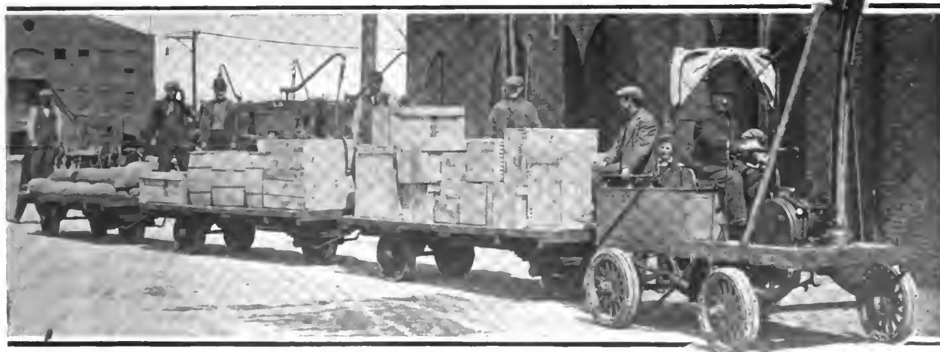
Battery crane truck for handling light freight at Bush Terminal. Giant warehouse in background
